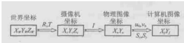
图 1 理想线性模型下的标定过程 Fig. 1 Process of calibration based on linear model
